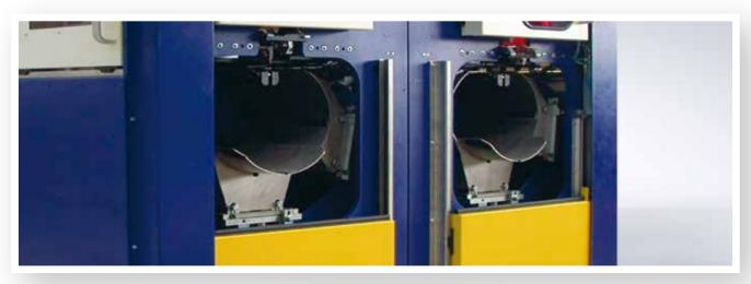
Economical one-station welding system for rings and parts with a diameter larger than part length
