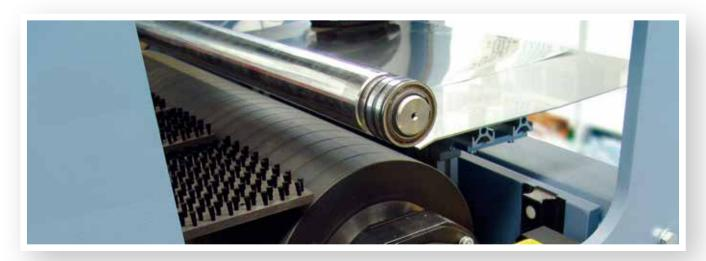
Automatic NC-controlled 2-roller rollformer suitable for integration in an automated production line
