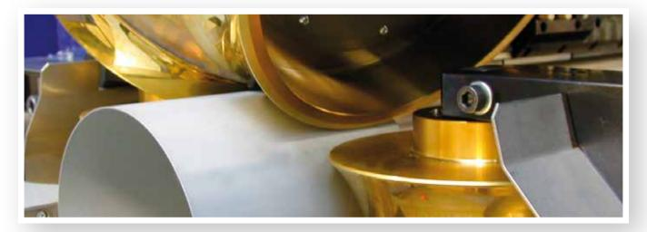
Production center for medium-sized short tubes with integrated Multiroller rollformer
