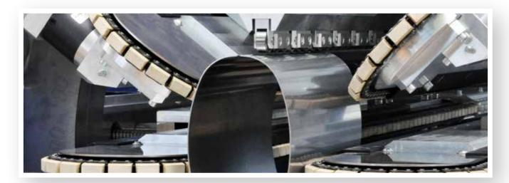
Innovative clamping technology for fully automatic production of round, oval and polygonal tubes.
