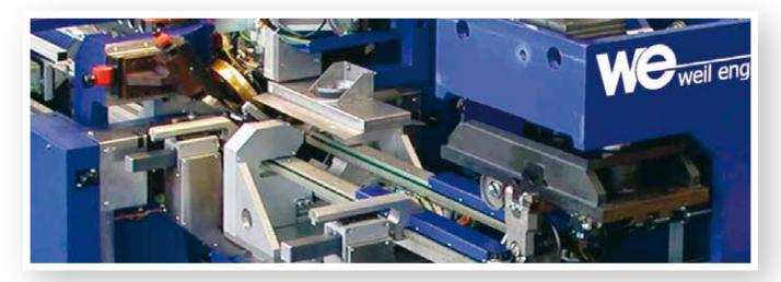
Continuous flow tube welding machine with high productivity and short cycle times
